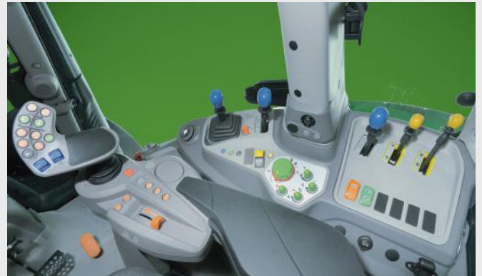
↑ RCshift: Available as a variant with mechanical control devices or as ↓ a variant with multifunction armrest, electro-hydraulic control valves and iMonitor.
