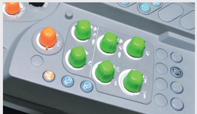
↑ The front linkage and rear linkage control can be fine adjusted with the potentiometers in the armrest.
