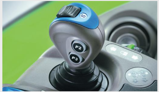
↑ The hydraulic valves are equipped with proportional control and can be fully programmed for time and quantity. The electronic joystick can be programmed to control the front loader, whereas other control valves can be operated using the thumbwheel.
