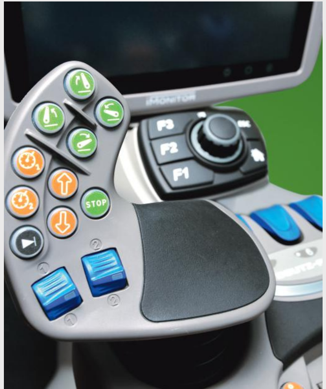
↑ With two buttons on the MaxCom multi-function joystick, the driver can use four different speed settings for field work or road application to maintain a constant speed for optimum results.
