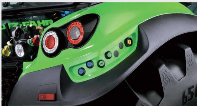
↑ Easy operation of the hydraulic system, rear linkage and PTO externally from both sides.
