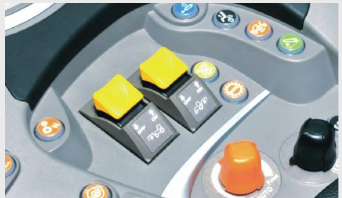
↑ The PTO control is easy and reliable to operate with a push button on all cab variants.
