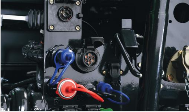
↑ The DEUTZ-FAHR ISOBUS interfaces at front and rear make the tractor compatible with attachments from all renowned manufacturers.
