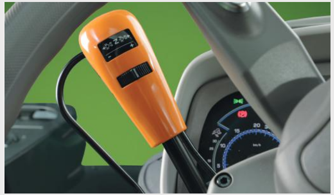
↑ PowerShuttle with Sense Clutch and five adjustment levels.
