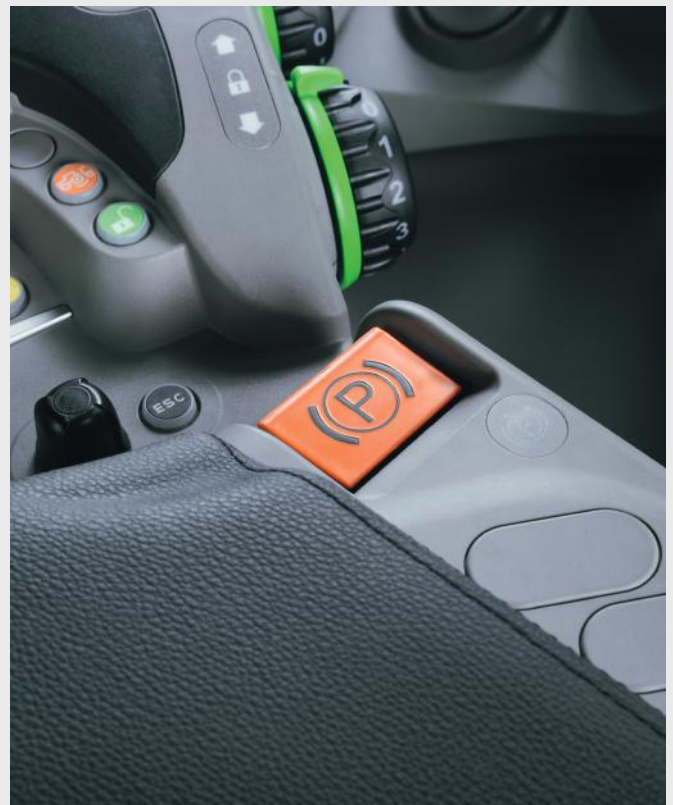
↑ On TTV models, the EPB replaces the mechanical handbrake lever and is operated via an electric push-button control on the armrest console.
