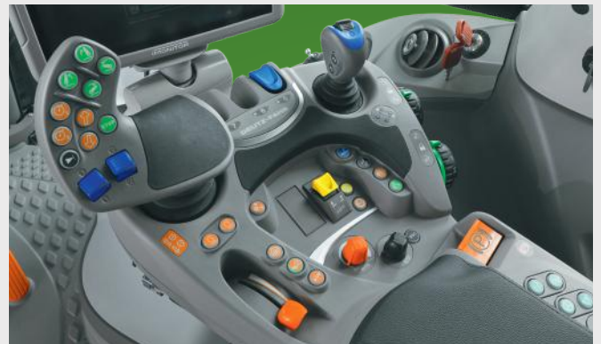
↑ TTV transmission: welcome to the premier league with optimum driving and operating comfort. Exclusively on TTV: position controlled front lift and electronic park brake integrated in the armrest.
