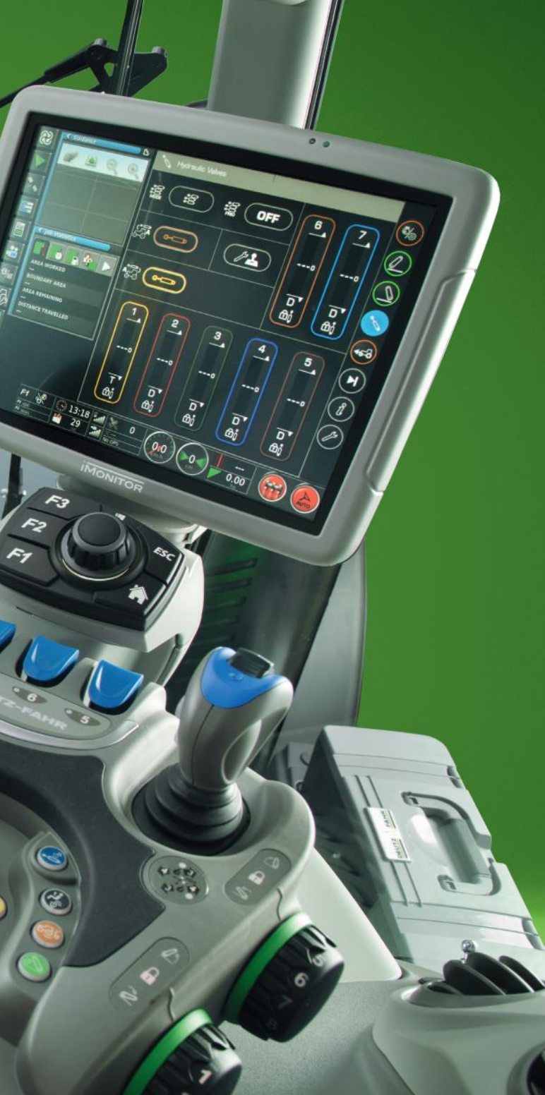
↑ The hydraulic valves are equipped with proportional control and can be fully programmed for time and quantity. The electronic joystick can be programmed to control the front loader, whereas other control valves can be operated using the thumbwheel.
