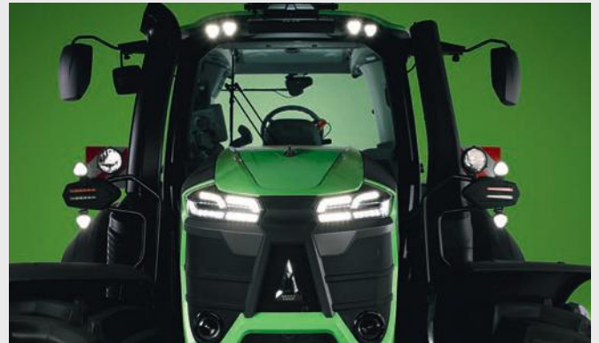
↑ LED package with up to 40,000 lm.
