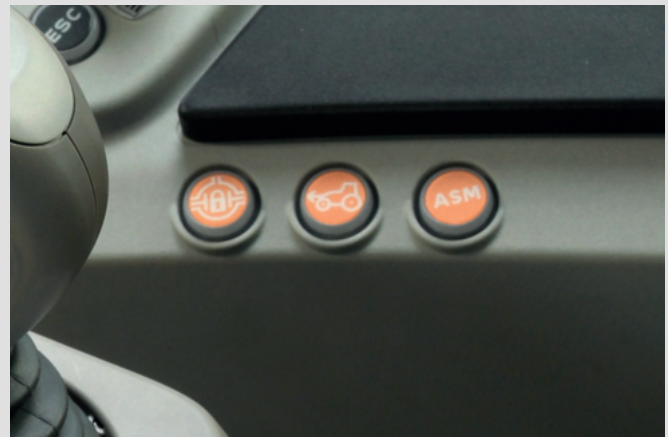
↑ Electrohydraulic front axle management.
