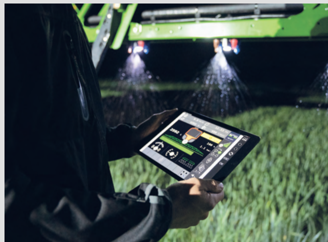
↑ XTEND function with tablet, control of implements via ISOBUS UT while being outside of the cab.
