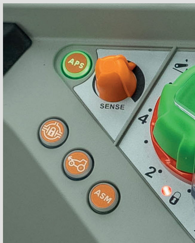
APS activation with adjustable response.
