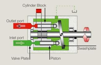
Unlike industry standards for this category of machines, Yanmar is using variable axial piston pump which adapt the flow and the pressure to the load, allowing smoother operation and improving the comfort of the operator. The pump flow of 2 x 11 l/mn and its high working pressure (210 bar) also enable to improve the productivity of the machine and its speed in working motion.
