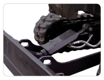
> The blade hydraulic cylinder is covered by a protective shield.
