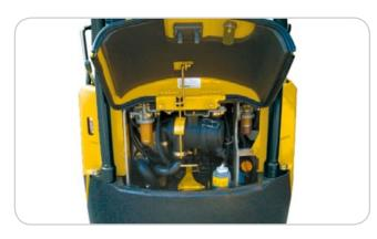
> Large rear bonnet allowing access to all engine components and hydraulic pumps.
